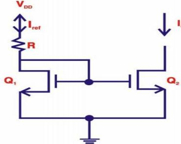
Let  $V_{DD} = 5V$ ,  $V_{TH,1} = 1V$ ,  $k_{n,1}' = 20 \mu A/V^2$  and  $R = 1K \Omega$ .
